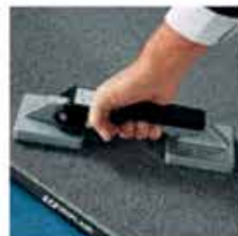
Lifting-tool with needles for carpet.
